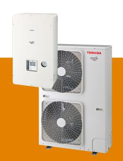
Air/Water heat pumps in a split design for flow temperatures up to +60°C, in the power levels of 8, 11, 14 kW, for generating hot or cold water. Combination of outdoor unit and hydro unit for supplying all applications such as hot water tanks, fan coils, radiators, or underfloor heating.
